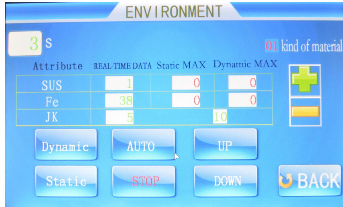
Environmental testing can be divided into two kinds of test method, which is used in the custom mode:conveyor running test or conveyor stopping test.
